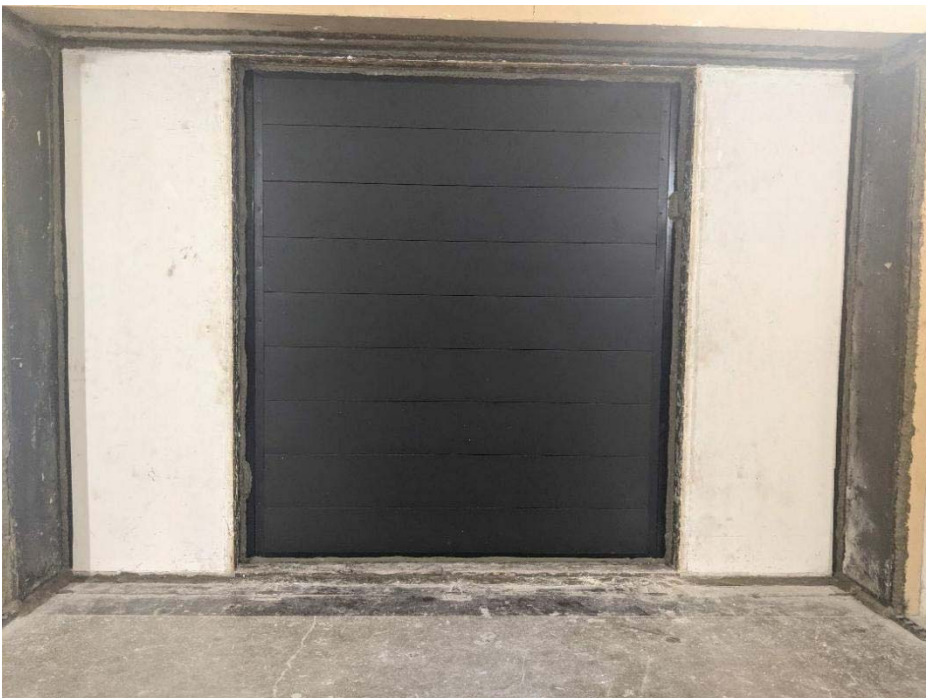
Figure 2 – Specimen mounted in test opening, as viewed from receive room
