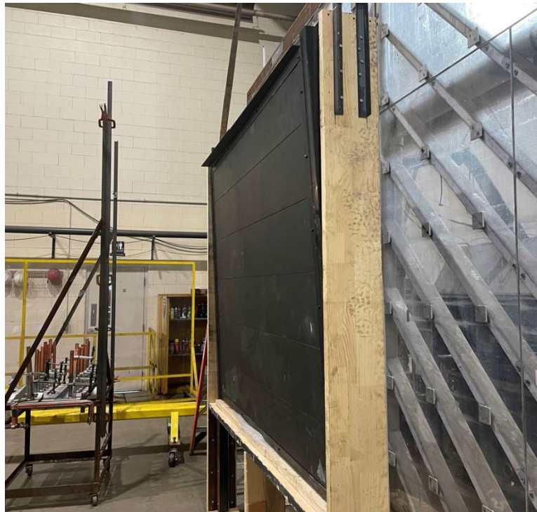
Photo #4: Permanent Set after 48 psf Load
